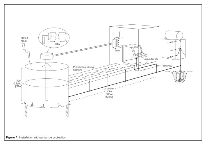
The diagram shows a two wire 4-20 milliamp transmitter with internal isolation fed from a galvanic isolator. To establish the order of the problem some assumptions are made which cannot be fully justified but are believed to be reasonable. These are:
