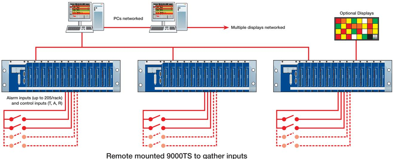
The System 9000TS is based on the standard eurorack, manufactured to IEC 297-3 (DIN 1494 Pt.5). The standard subrack size is 3U and 84E wide (19in).
