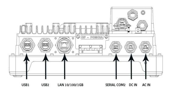
Figure 1 - Connector Layout – Workstation
