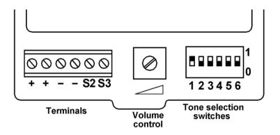
Figure 4 - Beka Horn internal power connection terminal
