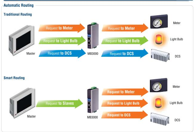
The MGate<sup>™</sup> MB3270, MB3280, and MB3480 include smart routing for enhanced compatibility with existing Modbus networks. Other Modbus gateways require a separate socket connection for each serial port, making them useless for TCP masters that can only open one connection. With smart routing on the MB3000 Modbus gateway, a TCP master can use just one socket connection to command serial slaves on every serial port.
