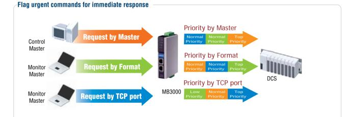
Other Modbus gateways simply transfer all requests between Modbus networks on a FIFO (first in first out) basis, with no accommodation for urgent commands that require immediate attention. The advanced models of the MGate™ MB3000 (the MB3170 and MB3270) include a patent-pending priority control feature that allows urgent commands to be flagged for immediate response based on IP address, command
