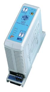
The MTL 9122-IS is a fieldbus repeater isolator which repeats the fieldbus signal from a safe area, Zone 2 fieldbus to an intrinsically safe fieldbus for connection to devices in Zone 1. The 9122-IS provides up to 265mA, typically powering up to 16 x 20mA field devices in Gas Group IIB.
