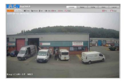
In the Live view interface, there are numerous operations like Snapping, Recording, Playback, Call, Listen, Clear Alarm, Log Search, Local Zoom of Image, Full-screen Viewing, PTZ and Lens Control.
