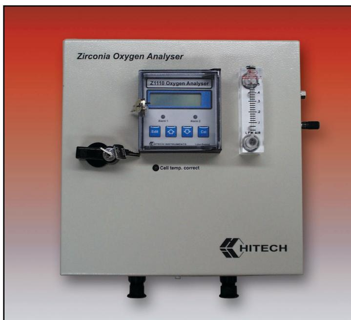
**The Z1110 zirconia oxygen analyser** measures oxygen concentrations from percentage levels to fractions of parts per million (ppm) in clean gases. Packaged in a robust wall mounting enclosure, it uses a zirconia oxygen sensor to provide accurate measurement with minimal interference from other gases. The unique cell and heater design gives a very fast warm-up time, rapid response, and long sensor life. A choice of sampling options is provided to produce virtually custom-built systems.
