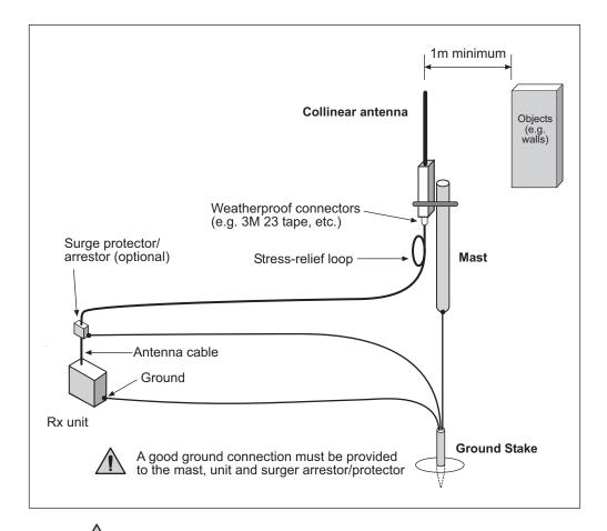
L The antenna must be be installed above all local obstructions
