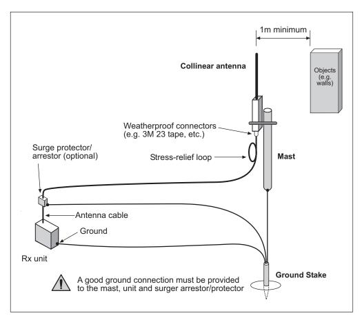
The antenna must be be installed above all local obstructions
