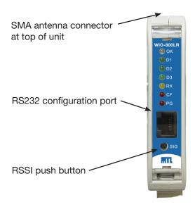
The LEDs on the front panel indicate the unit status:
