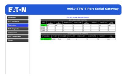
• This page shows the counters for all of the LAN connected Modbus/TCP clients as well as the serial ports, this can be useful for fault finding
