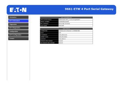
This shows information about the Wi-Fi module and the current settings associated with it, including whether there is an active Wi-Fi connection.
