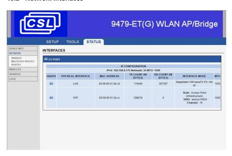
This Page shows a summary of the currently configured network interfaces and displays the transmitted and received packets.
