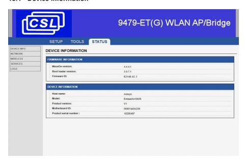
The Device Information page allows a quick overview of the unit's useful information and the currently installed firmware information.
