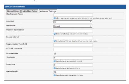
**Max Transmit Power:** The transmit power is normally set automatically based on the regulation rules for the given channel and the capabilities of the radio card. This option sets an upper bound on the transmit power. The transmit power is distributed between the configured antennas.
