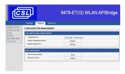
The Save and restore configuration section allows you to backup the units current settings to a file. You are then able to restore the previously saved file, back into the unit. This will load up all of its previous settings
