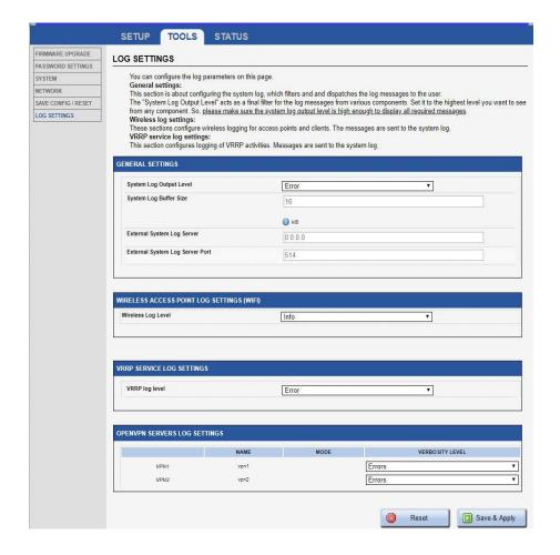
This is the log settings page, it allows you to configure the system logs.
