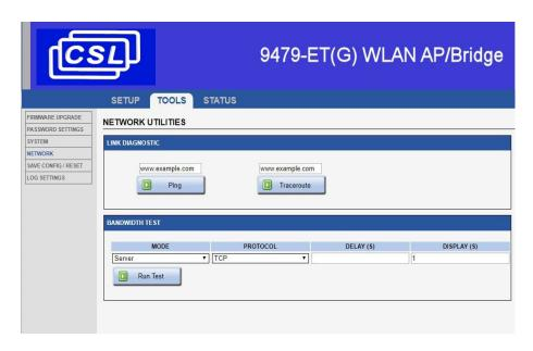
This panel provides two standard UNIX tools: ping and traceroute. Place the argument in the text field above the corresponding button and then click the button. The results will be displayed in a frame below.
