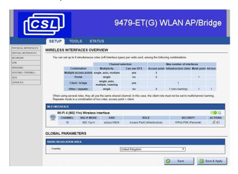
This page allows the user to configure the wireless network settings, by default the radio will be disabled and you will need to turn in on.
