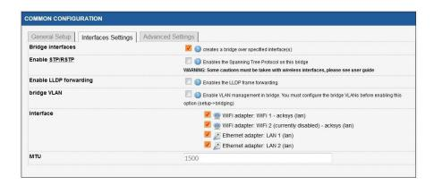
**Bridge Interfaces:** If checked, all interfaces in this network are linking with the software equivalent of an Ethernet switch.
