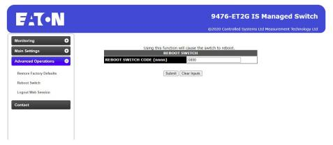
This page allow the rebooting of the unit. To reset enter the reboot device code.
