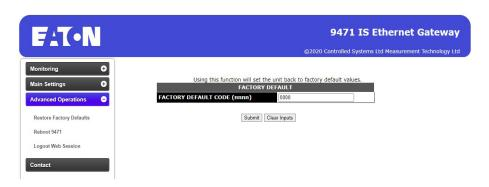
This page allow the resetting of the unit back to Factory Defaults. To reset enter the factory reset code .
