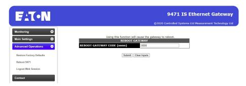
This page allow the rebooting of the unit. To reset enter the reboot device code.
