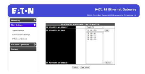
The Web page above accessed via password allows the user to configure a whitelist of IP addresses. The IP Whitelist is a feature that allows the user to specify what IP Addresses can communicate Modbus through the 9471.
