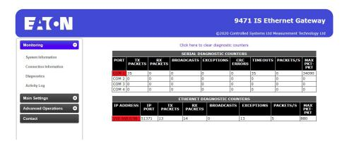
This page shows the counters for all of the LAN connected Modbus/TCP clients as well as the serial ports, this can be useful for fault finding on the network.
