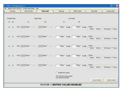
On the above screen the rates can be set in Mbps for both low and high priority messages. To limit High priority messages ensure the Disable Priority check boxes are not selected. The rate limits can be enabled by selecting the check boxes on the appropriate limit. The priority for each port can be set to be Diffser, 802.1P, Port Based or None.
