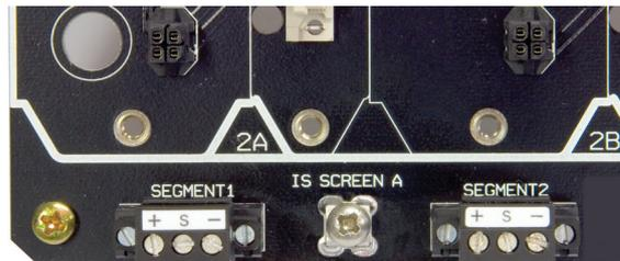
The intrinsically safe segment power output connections are provided via 3-way, pluggable, rising cage clamp, screw terminals at the bottom edge of the 9107-22 module carrier. See Figure 4.3.
