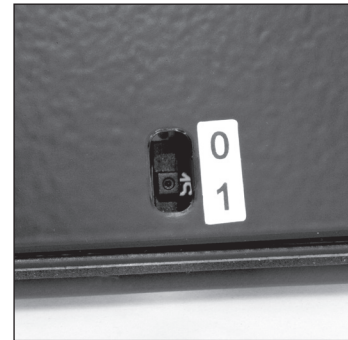
Figure 2-7: Ground reference switch set to '1'
