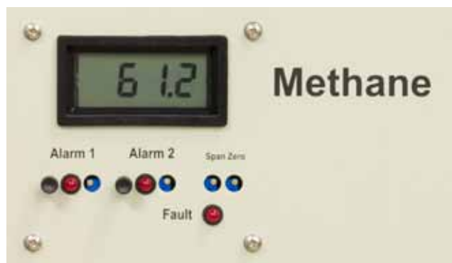
Figure 1 - Typical gas display showing Alarm setting facilities, Span and Zero adjustments and a Fault indicator.
