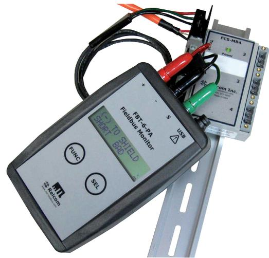
device on the segment is displayed in turn by pushing the "SELECT" button. The first device shown will be the Master. By default, measurements greater than 150mV are OK. If a device leaves the segment, a "-" is displayed; if a device is added it shows "+".
