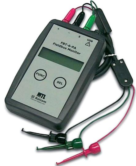
**The Profibus-PA Diagnostic Monitor, FBT-6-PA,** is used to examine the operation of a live Profibus-PA segment without interfering with its operation. The Monitor is intended for maintenance personnel to verify segment operation or to troubleshoot an errant segment.
