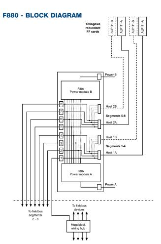
The above diagram shows a block diagram of how the F880-CA-RT is wired. Note that the Chassis Ground and Alarm connection are not shown. The Diagnostic module is also not shown (see the F809F product specification).
