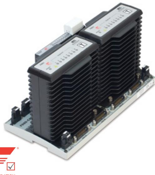
The **F880 fieldbus power system** is designed to provide redundant power for eight FOUNDATION™ fieldbus H1 segments when used with Yokogawa ALF111 fieldbus cards. The F880 module carrier has system connectors for direct connection to two redundant pairs of fieldbus cards using Yokogawa AKB336 cables.
