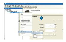
Also, the current values and alarm limits can be exported and it is normal practice to save a baseline of data as part of the commissioning procedure. The F809F DTM compare function will allow a comparison of the current values against the start up baseline or any other dataset.
