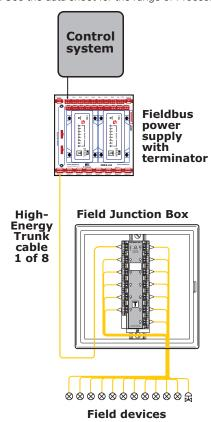
Shown above is an example of a common Fieldbus segment topology. Twelve field devices are connected to a twelve-drop Megablock, which is mounted in a field junction box. The trunk connector on the Megablock is wired to the segment trunk cable that leads to the control room or marshalling panel where the power supply and second terminator are located.
