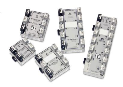
Megablocks are DIN-rail mounted passive hubs for FOUNDATION™ fieldbus networks. They connect several field devices to the network trunk cable and provide short circuit protection to the segment. Megablocks minimize hand wiring and allow individual devices to be added to and removed from the segment without disrupting network communication.
