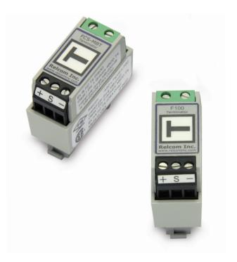
**The fieldbus standards** require that buses must be terminated at both ends to prevent signal reflections. Usually one terminator is provided by the power conditioner in the control room. The MTL range of fieldbus terminators are ideally suited to provide the Terminator that is normally in a junction box in the field (along with a Megablock for interconnecting devices). A large "T" is placed on all terminator labels for easy identification of the Terminator location.
