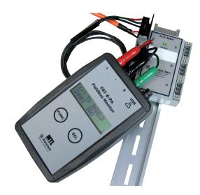
device on the segment is displayed in turn by pushing the "SELECT" button. The first device shown will be the Master. By default, measurements greater than 150mV are OK. If a device leaves the segment, a "-" is displayed; if a device is added it shows "+".
