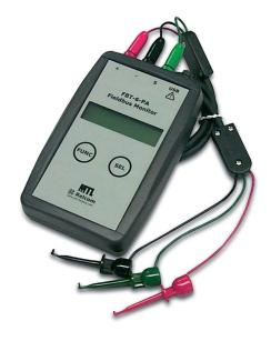
**The Profibus-PA Diagnostic Monitor, FBT-6-PA,** is used to examine the operation of a live Profibus-PA segment without interfering with its operation. The Monitor is intended for maintenance personnel to verify segment operation or to troubleshoot an errant segment.
