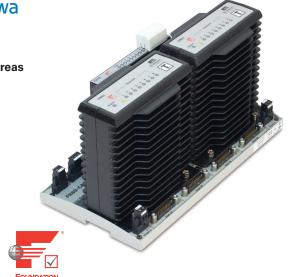
The F880 fieldbus power system is designed to provide redundant power for eight FOUNDATION™ fieldbus H1 segments when used with Yokogawa ALF111 fieldbus cards. The F880 module carrier has system connectors for direct connection to two redundant pairs of fieldbus cards using Yokogawa AKB336 cables.
