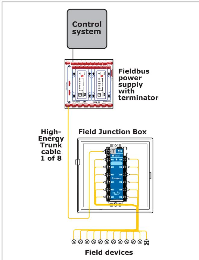
Shown above is an example of a common Fieldbus segment topology. Twelve field devices are connected to a twelve-drop Megablock, which is mounted in a field junction box. The trunk connector on the Megablock is wired to the segment trunk cable that leads to the control room or marshalling panel where the power supply and second terminator are located.
