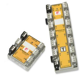
Megablocks are DIN-rail mounted passive hubs for Foundation<sup>™</sup> fieldbus networks. They connect several field devices to the network trunk cable and provide short circuit protection to the segment. Megablocks minimize hand wiring and allow individual devices to be added to and removed from the segment without disrupting network communication.
