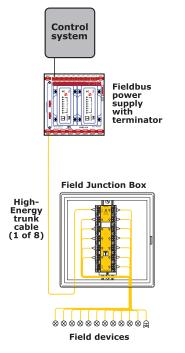
Shown above is an example of a common Fieldbus segment topology. Twelve field devices are connected to a twelve-drop Megablock, which is mounted in a field junction box. The trunk connector on the Megablock is wired to the segment trunk cable that leads to the control room or marshalling panel where the power supply and second terminator are located. The example shows the increased safety (Ex em) version connected to a general purpose fieldbus power supply.
