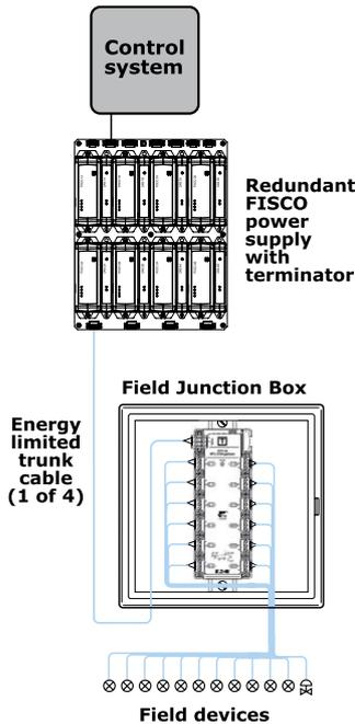
Shown above is an example of a common Fieldbus segment topology. Twelve field devices are connected to a twelve-drop Megablock, which is mounted in a field junction box. The trunk connector on the Megablock is wired to the segment trunk cable that leads to the control room or marshalling panel where the IS power supply and second terminator are located.
