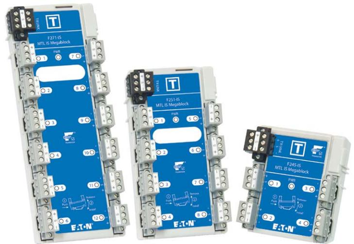
The **F2xx-IS MTL Intrinsically Safe (IS) Megablocks** are DIN-rail mounted passive hubs for Foundation™ fieldbus networks. They connect several IS field devices to the network IS trunk cable and provide short circuit protection to the segment. Megablocks minimize hand wiring and allow individual IS devices to be added to and removed from the segment without disrupting network communication.
