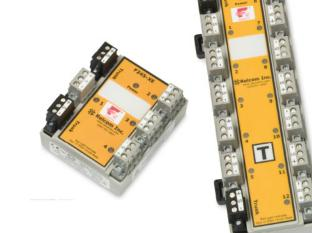
**Megablocks are DIN-rail mounted passive hubs** for Foundation<sup>™</sup> fieldbus networks. They connect several field devices to the network trunk cable and provide short circuit protection to the segment. Megablocks minimize hand wiring and allow individual devices to be added to and removed from the segment without disrupting network communication.
