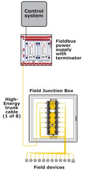
Shown above are examples of common Fieldbus segment topologies. Twelve field devices are connected to a twelve-drop Megablock, which is mounted in a field junction box. The trunk connector on the Megablock is wired to the segment trunk cable that leads to the control room or marshalling panel where the power supply and second terminator are located. The example shows the increased safety (Ex em) version connected to a general purpose fieldbus power supply.
