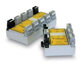
AS-i Megablocks are DIN-rail mounted passive\* hubs for the AS-i network. They connect several AS-i devices to the network trunk cable and provide short circuit and over voltage to the segment. The AS-i Megablock itself does not contain an AS-i chip or communicate over the AS-i network, so it consumes no network communication resources (bandwidth, slave addresses, etc.). They are used to interconnect AS-i master and slave devices that do contain AS-i chips.
