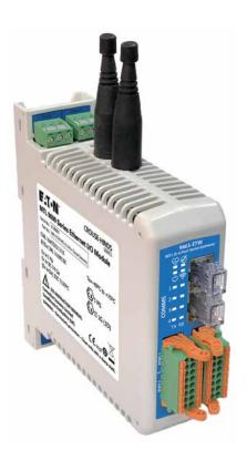
The 9661-ETW is an MTL Intrinsically Safe (IS) Ethernet to Serial 4 Port Communication Module suitable for Zone 1 mounting with a suitable Ex ib power supply, Zone 0 with a suitable Ex ia power supply.
