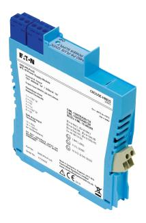
The MTL 9492-PS-PLUS power supply is the preferred method for supplying the 9460-ET series of intrinsically safe ethernet modules and is based on an isolating power supply. It takes a 24V DC safe area / Zone 2 supply and produces an intrinsically safe, 12V DC nominal output capable of powering the ethernet modules mounted in a Zone 1 hazardous area. The 9492-PS-PLUS may be mounted in a safe area or Zone 2 hazardous area.
