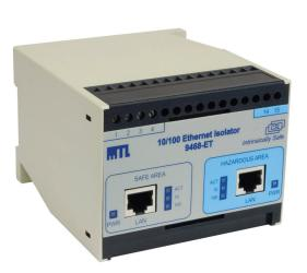
The 9468-ET 10/100Mbps, Isolating Ethernet Barrier allows the interconnection of a Zone 2 or uncertified safe area device to the intrinsically safe 9400-ET range of Ethernet networking products, operating in the hazardous area.
