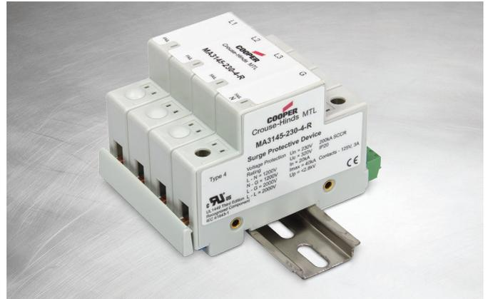
The MA3100 Series offers cost effective, DIN-rail mounted, surge protection for applications described by IEC 61312. The Class II range of surge arrestors fit in to the cascade philosophy along side Class I & Class III devices.
