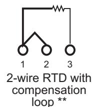
\*\* The multiplexer must be configured for a 3-wire RTD in order to recognise an RTD with a compensation loop.
