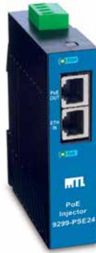
The 9299-PSE24A/B or 9299-PSE48A/B industrial PoE power injectors add 48V DC power into one or two Ethernet ports so that both power and data can be passed over the same wire to Ethernet devices in the field. The PSE24A/B models step up a 24V DC source to power a single PoE port, avoiding the need for a separate DC/DC converter. The PSE48A/B models provide two injectors in one package to save both space and money. Both models are ultra-rugged, reliable and easy to use.
