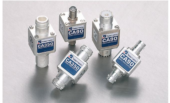
The CA range of surge protection devices prevents surges and transient over-voltages conducted through coaxial cables from damaging electronic systems such as telemetry outstations. They protect vulnerable equipment without affecting normal operation, passing high frequency signals with little attenuation while diverting surge currents safely to earth and clamping output voltages to safe levels.
