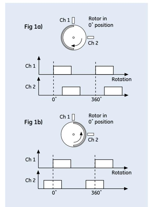
The second channel can be used to determine direction of rotation by comparing the phase of its input pulse with that of the first channel.
