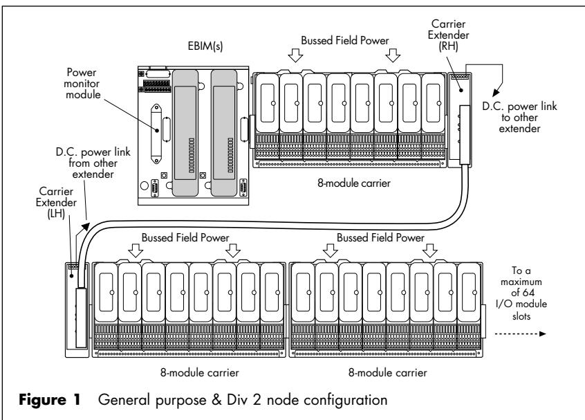
**Figure 1** General purpose & Div 2 node configuration
