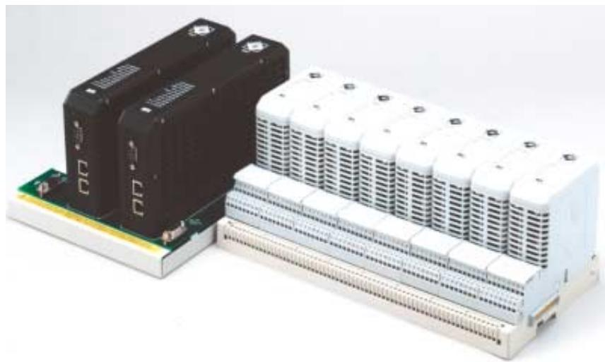
can be set to maintain last value or drive to a specific value (e.g. high or low when fail safe mode is adopted). In the event of power loss, the EBIM will perform a cold restart, which restores the system to a pre-defined status.
