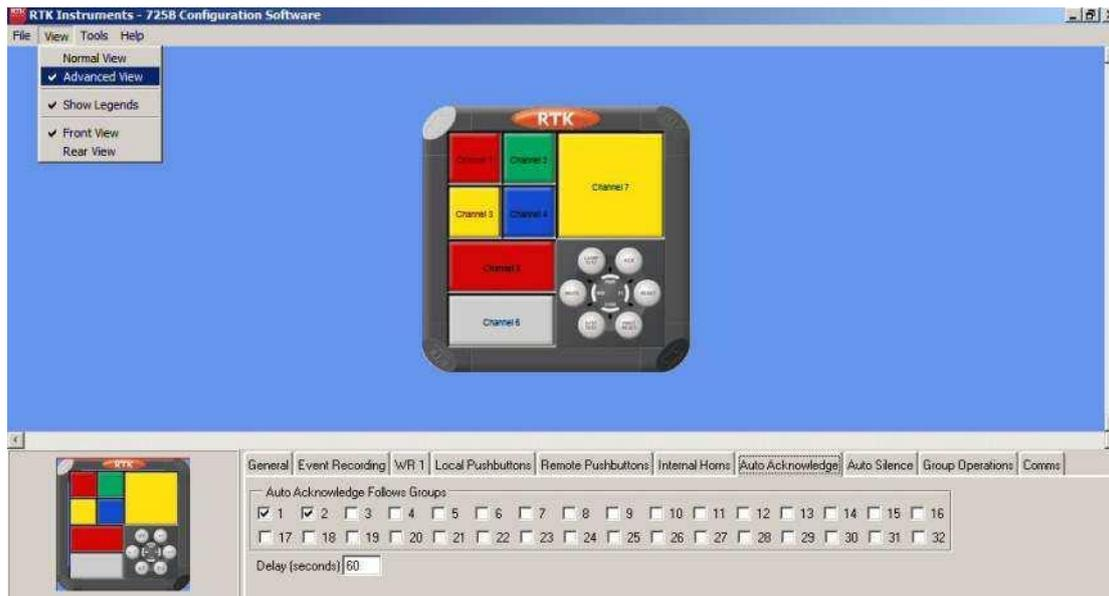
Note: On systems supplied after 1st February 2010 using configuration software version 2.0.8 or higher the Auto Acknowledge operates the Acknowledge group 2 pushbutton, as this allows you the flexibility to pick which channels to auto acknowledge. To set a channel to auto acknowledge it must be put into Acknowledge Pushbutton group 2 using the pushbutton group 2 using the pushbutton group tab on the individual channel.
