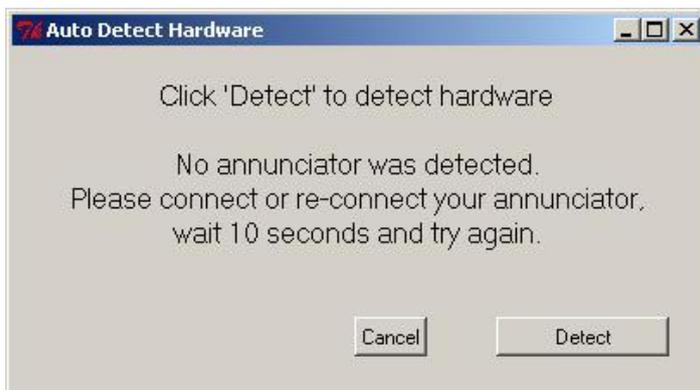
If any conflicts are found during the detection process an error message will provide diagnostic details to assist the user with fault finding.
