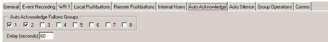
Once set the system will automatically acknowledge the alarms associated with the selective group after the preset time period has elapsed.
