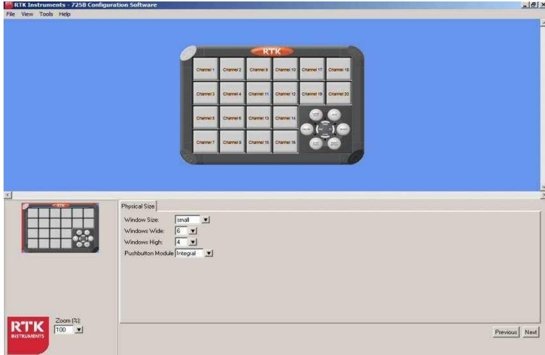
To enable the integral pushbutton function the drop down menu to the right of the “Pushbutton Module” field needs to be selected to Integral.
