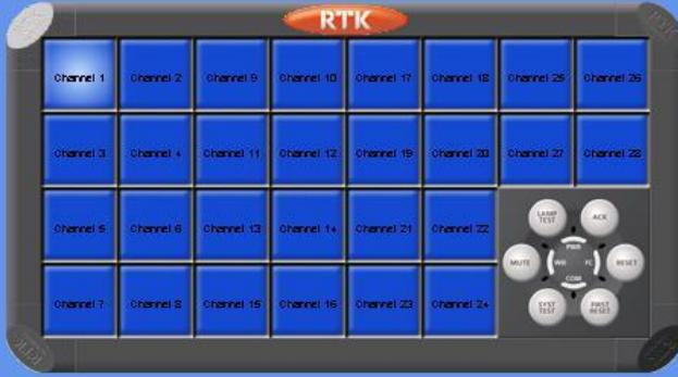
The image shows a physical RTK 725B annunciator panel. It features a grid of 28 blue pushbutton channels labeled Channel 1 through Channel 28. To the right of the grid is a cluster of control buttons: LAMP TEST, ACK, MUTE, SILENCE, and RESET. The panel is mounted on a blue background.
