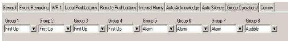
To prevent the audible sounding on a status window the user should select a single status alarm window or group of status alarm windows and uncheck the tick box associated with a Group being used as an Audible in the example above this would be Group 8
