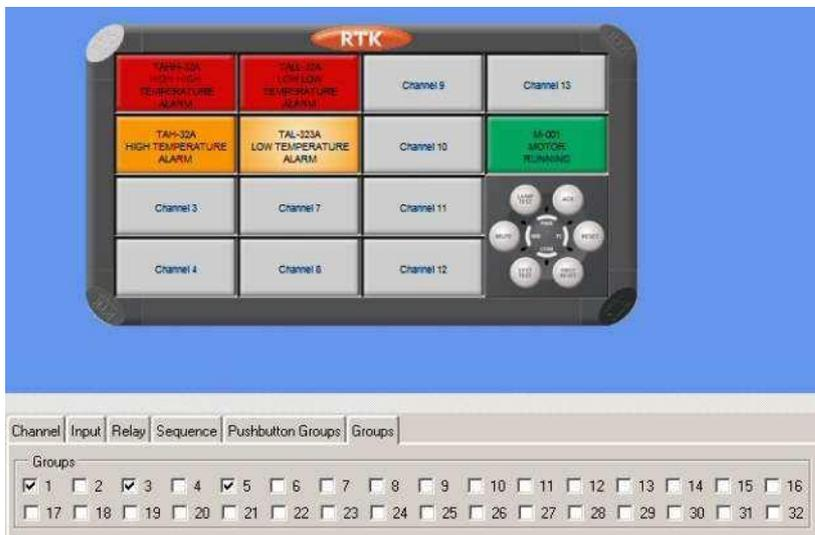
In the example shown above Channel 6 has been assigned to Horn Group 1, 3 & 5. Once a Horn Group has been defined the user can assign a single or multiple Relays to any of the Groups as detailed under the “WR1” Watchdog / Relay Tab Setting within this manual.
