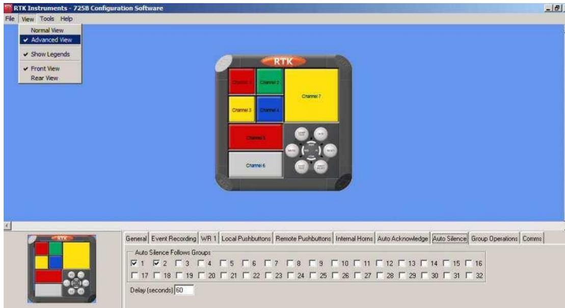
Note: On systems supplied after 1st February 2010 using configuration software version 2.0.8 or higher the Auto silence operates the silence group 2 pushbutton, as this allows you the flexibility to pick which channels to auto silence. To set a channel to auto silence it must be put into silence Pushbutton group 2 using the pushbutton group tab on the individual channel.
