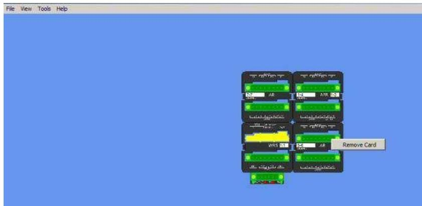
Once a card has been removed in software the associated terminal view changes to yellow from green to indicate that the card is no longer present.
