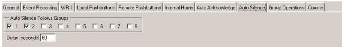
Once set the system will automatically Silence the alarms associated with the selective group after the preset time period has elapsed. Please note: This feature only Silences the audible alarm, the visual alarm will continue to operate in accordance with the selected ISA sequence.
