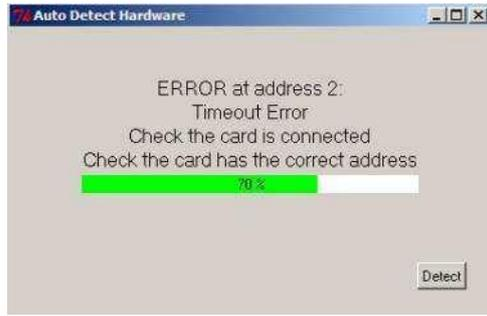
In this example the card set to address 2 has not been successfully detected and the auto detect halts until the user resolves the issue
