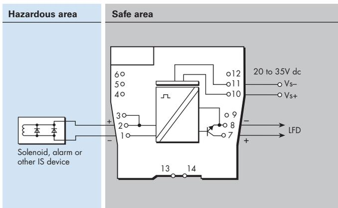
Red: LFD indication, on when line fault detected
