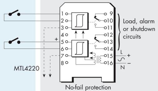
All contacts shown in alarm condition (relay de-energised)
