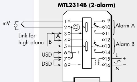
All contacts shown in alarm condition (relay de-energised)
