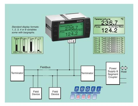
The BA688CF-P Fieldbus Display is a general purpose instrument that can display up to eight fieldbus process variables. Eleven selectable standard screen formats contain one, two, three, four or eight variables, with units of measurement, tag descriptions and bargraphs on some screens.
