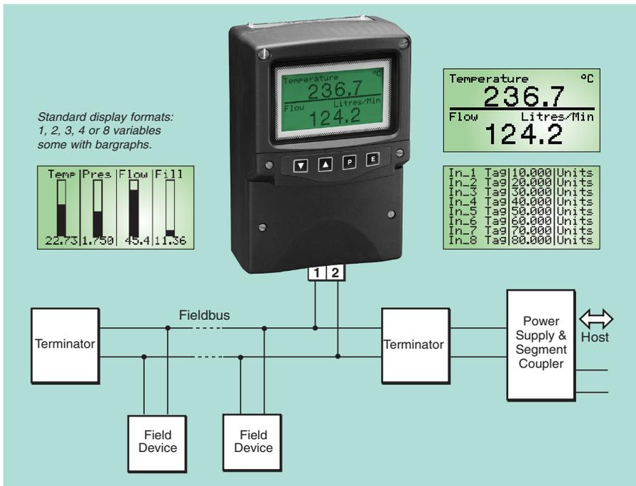
The BA684DF-P Fieldbus Display is a general purpose instrument that can display up to eight fieldbus process variables. Eleven selectable standard screen formats contain one, two, three, four or eight variables, with units of measurement, tag descriptions and bargraphs on some screens.
