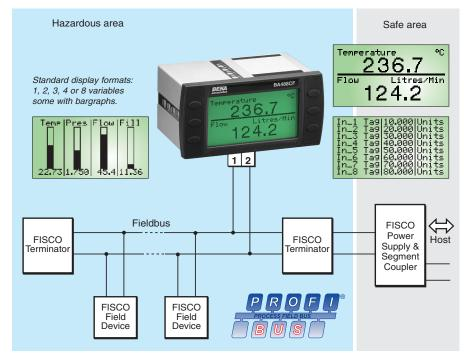
The BA488CF-P Fieldbus Display is an intrinsically safe instrument that can display up to eight fieldbus process variables. Eleven selectable standard screen formats contain one, two, three, four or eight variables, with units of measurement, tag descriptions and bargraphs on some screens.
