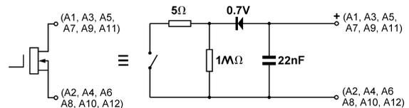
Fig 4 Equivalent circuit of each switch output
