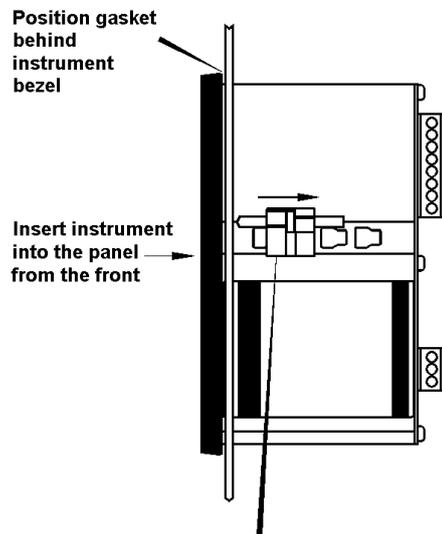
Slide panel mounting clip into the slotted rail on the side of the enclosure. Four clips are required to achieve an IP66 seal between instrument and panel.
