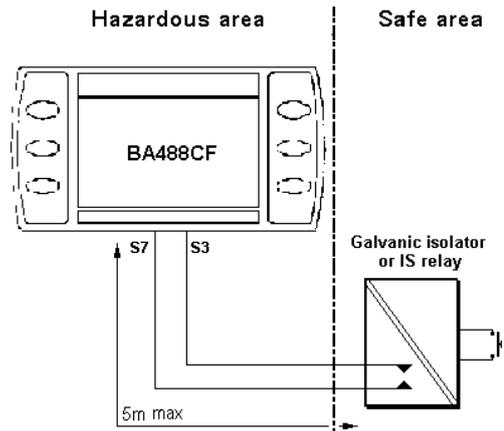
Fig 3 External push button switch in safe area
