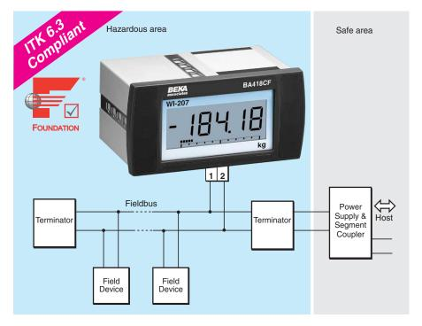
The BA418CF-F Fieldbus Indicator is a cost-effective intrinsically safe panel mounting instrument that displays a single fieldbus process variable in a hazardous area. Housed in a robust panel mounting enclosure with an IP66 front, the instrument has a large, high contrast five digit display and a horizontal bargraph. The BA418CF-F indicator uses the same technology and compliments the well established BEKA eight variable fieldbus displays that are now in worldwide use.
