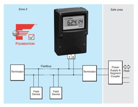
The BA414NDF-F Fieldbus Display is a new cost-effective Type nL field mounting instrument that can display a single fieldbus process variables in a Zone 2 or Zone 22 hazardous area. Housed in a robust IP66 GRP enclosure, the instrument has a large, high contrast five digit display, plus a horizontal bargraph. The BA414NDF-F uses the same technology and compliments the well established BEKA eight variable fieldbus displays that are now in worldwide use.
