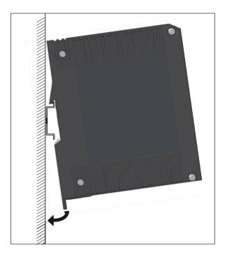
You have the option of attaching the device to a vertical flat surface. This requires a wall mounting plate, which you purchase as a separate accessory.
