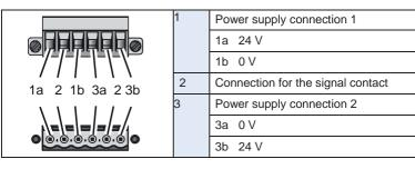
Table 6 - Pin assignment: 6 pin, screwable terminal block (on the top), connection to the device (at the bottom)
